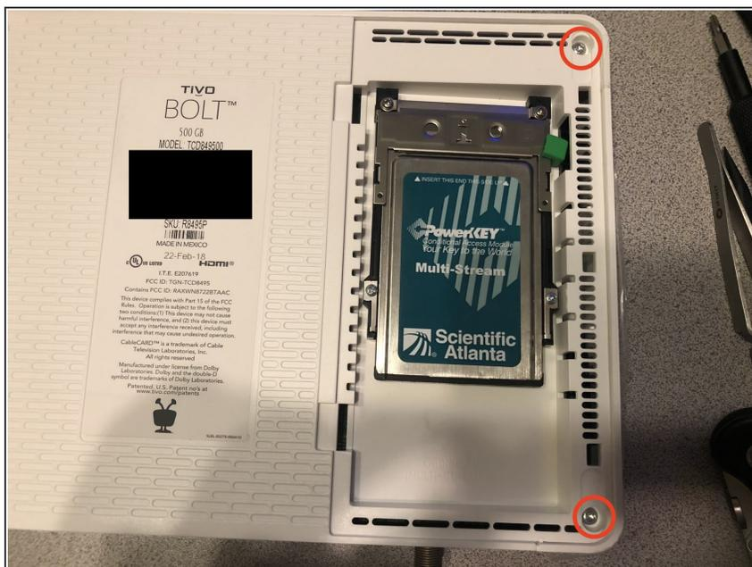
**⚠** Do not attempt to remove the housing yet. Still 3 more screws and plastic clips holding it in place
