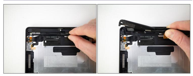
• Pry up the left speaker with the flat end of a spudger and remove.
