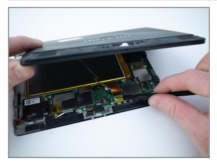
• Use the flat end of a spudger to pry up and disconnect the rear panel press-fit connector from the motherboard.
