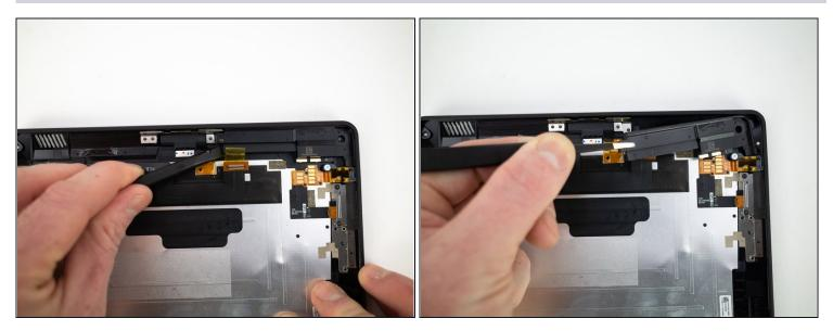
• Pry up the right speaker with the flat end of a spudger and remove.
