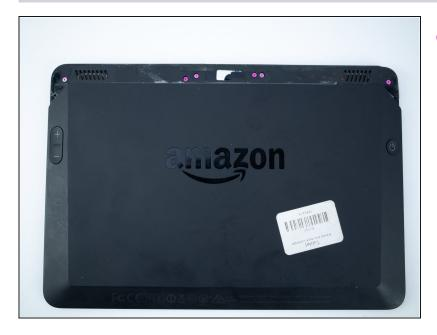
• Remove the six pink 3mm T3 Torx screws from the back case.
