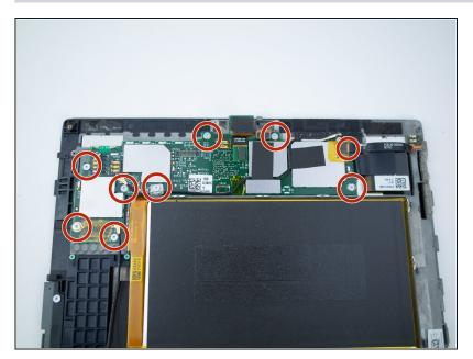
• Remove the nine 3mm T6 Torx screws from the motherboard.
