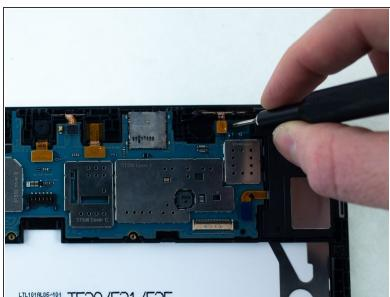
Remove the two 2.7mm Phillips #00 screws from the motherboard.
