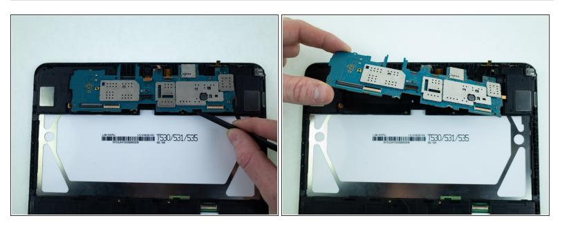
Use a spudger to pry up the motherboard, and remove it from the device.
