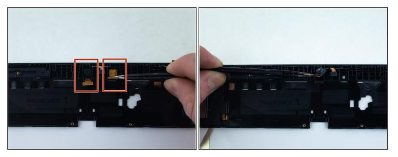
Pull up on the cameras with a pair of tweezers to remove.
