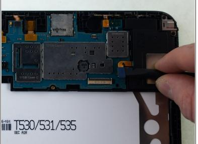
Use the flat end of a spudger to pry up and disconnect the five press-fit connectors from the motherboard.
