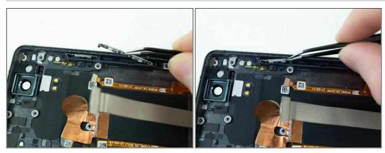
• Remove the remaining button halves with a pair of tweezers.
