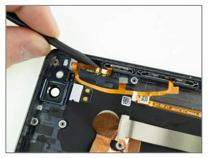
Use the pointed end of a spudger to gently lift up the button ribbon cable from the phone.
