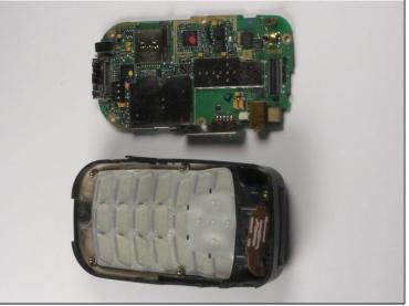
Remove the logic board from the anterior piece of the outer case using the plastic opening tool.
