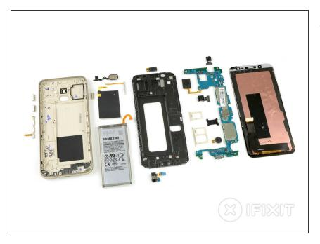
This completes our abbreviated teardown, with all components lined up for inspection. We'd hoped for a bit more modularity in this mid-range phone—but let's tally up the points and see how the J6 performed.
