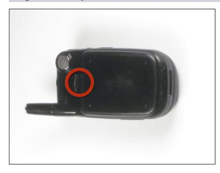
Push the highlighted button in the direction in which the antenna is pointing. The battery will release and pop up.
