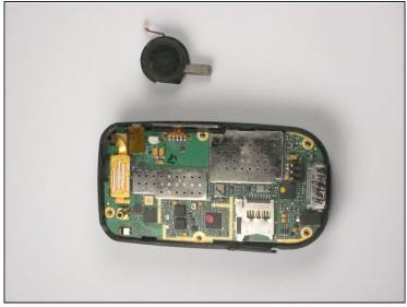
• Remove the wire attached to the speaker from the motherboard using tweezers.
