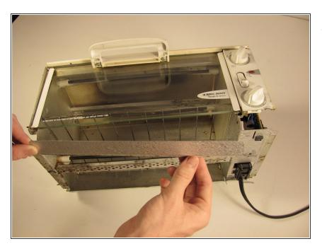
Remove the aluminum strip on the bottom of the unit.
