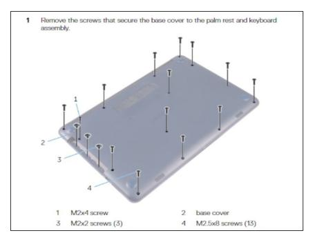
Put the base cover back on the laptop and do the reverse of step 1.
