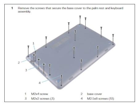
Remove the screws that secure the base cover to the palm rest and keyboard assembly.
