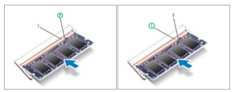
Align the notch in the NEW memory module with the tab in the memory module connector.
