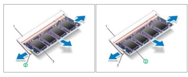
Use your fingertips to carefully spread apart the securing clips on each end of the memory module connector until the module pops up.
