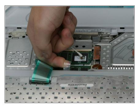
Pull up the keyboard connector cable by its clear plastic loop.
