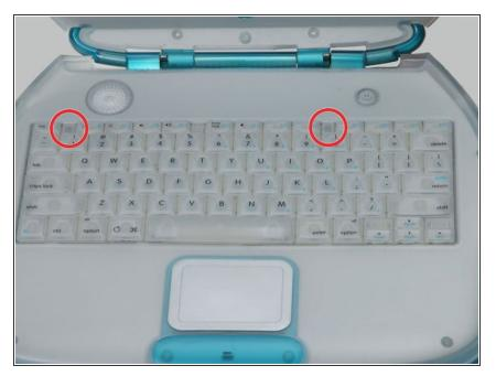
Pull the keyboard release tabs toward you and lift up on the keyboard until it pops free. Note that the keyboard ribbon is still attached to the logic board, so you cannot completely remove the keyboard yet.
