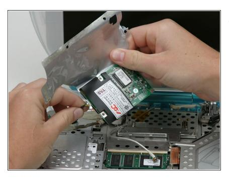
Lift the modem partially out and disconnect the cable on the left side.
