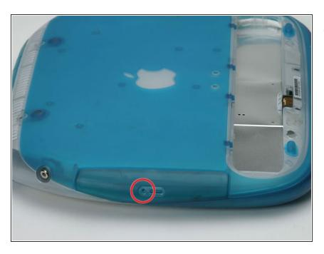
Use a straightened paperclip to manually eject the CD-ROM tray.
