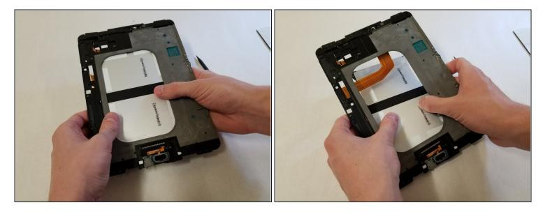
• Flip the midframe over and pop the battery out, making sure to slide it out from underneath the ribbon cables.
