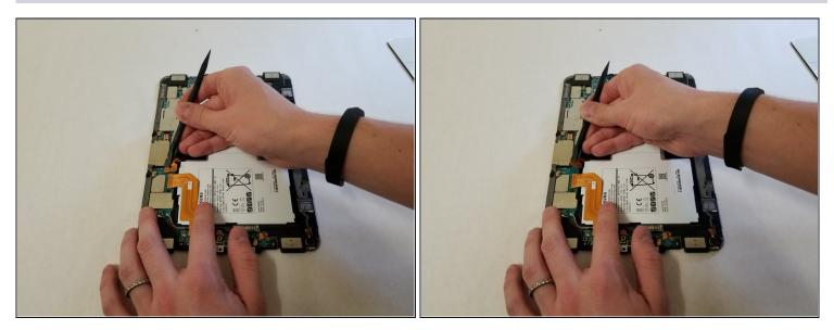
• Use the flat end of the **spudger** to pop off the connector between the battery and the motherboard.
