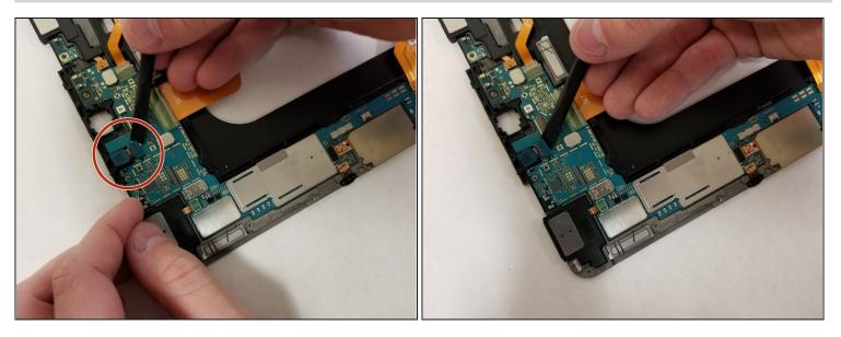
• Carefully pop the front facing camera off from the motherboard with the flat end of the **spudger**.
