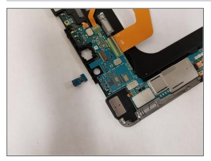
• Remove the front facing camera from the device.
