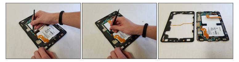
• Locate the ribbon running from the midframe and disconnect it from the motherboard with the flat end of a **spudger**.
