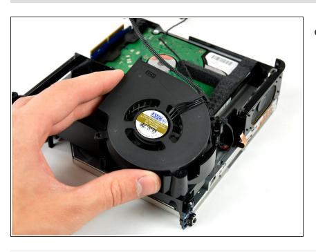
Lift the fan out of the internal frame, minding any cables that may get caught.
