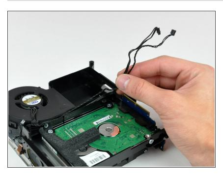
De-route both the fan and IR board cables out of the channel in the internal frame.
