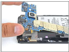
Holding the motherboard by the top corners, hinge it upwards while clearing flex cables out of its path.
