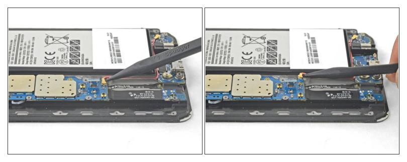
Using the pointed end of a spudger, disconnect the antenna cable.
