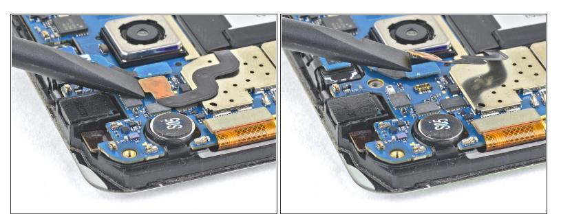
Using the flat end of a spudger, lift the battery connector straight up from its socket on the motherboard.
