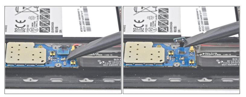
Using the flat end of a spudger, disconnect the navigation buttons connector.
