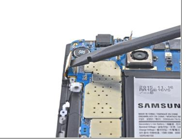
Using the flat end of a spudger, disconnect the display connector.
