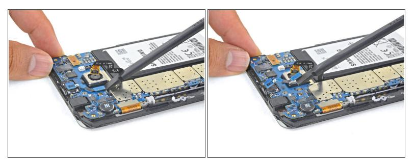
Using the flat end of a spudger, disconnect the earpiece connector.
