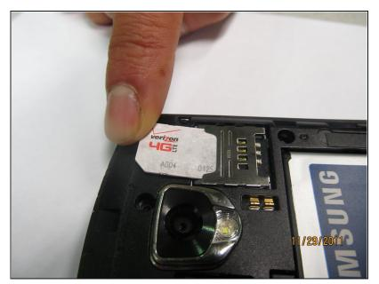
Slide the SIM card out of its casing by pushing on it and sliding it upward.
