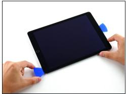
• Slide the left-hand opening pick along the bottom edge of the display, then remove it from the bottom right corner of the iPad.
