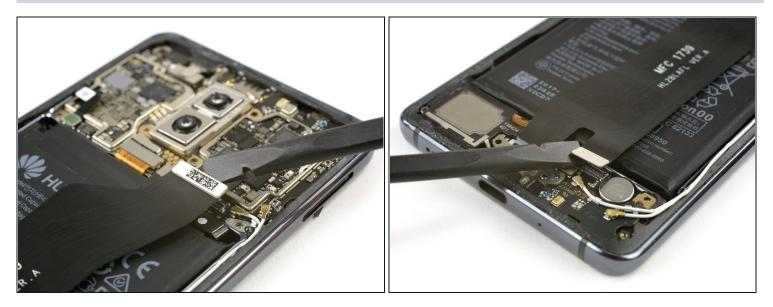
• Use a spudger to disconnect the charging port flex cable from the motherboard and from the daughterboard.
