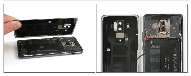
⚠ Don't remove the back cover all the way, yet. The fingerprint sensor cable is still connected to motherboard.
