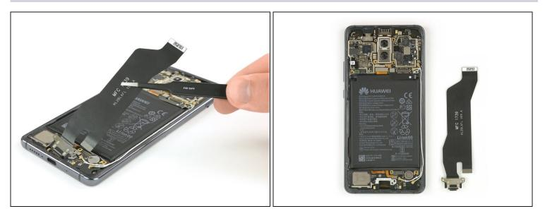
Use a pair of <u>tweezers</u> to carefully remove the charging port including its flex cable.
