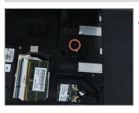
Use a PH0 screwdriver to remove the single screw holding in the optical drive.
