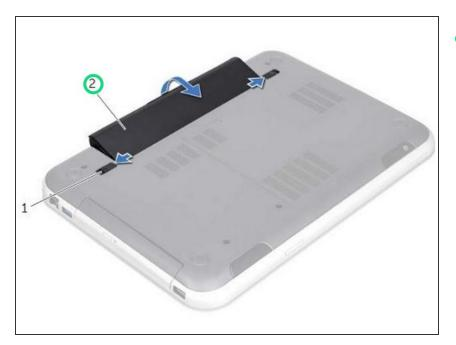
Lift the battery out of the battery bay.
