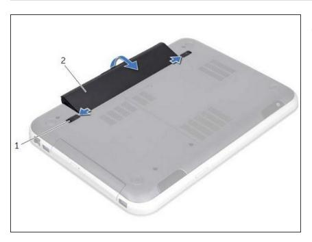
Align the tabs on the NEW battery with the slots on the battery bay and snap the battery until it clicks into place.
