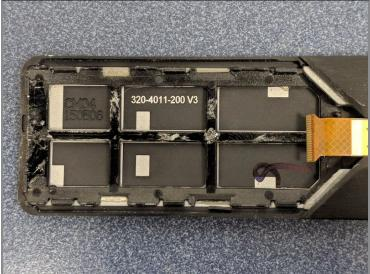
• Once you have the Circuit out of the glue you will see the shown Ribbon attachment clip moved up to be removed. Second picture the board is removed.
