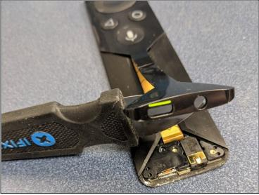
• From here you will want to use the Jimmy or similar item to get under the bottom corner to get past the inner clips. From here you can carefully get both sides of the bottom top cover and lift it off. The remainder of the cover should come off fairly easily. If not use the jimmy to unclip the others.
