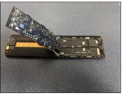
• Use the Jimmy to prop the circuit board from the glue attached to the casing. Becareful of the ribbon attached. The circuit board will come out away from the ribbon if you remove it from the glue.
