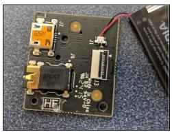
• From here you can remove the Single Phillips Screw using the Phillips 00 Driver Bit. This will let you pry the circuit and battery from the Glue. You can lift the Battery from the Circuit board as it is made to lift upward and away from the board.
