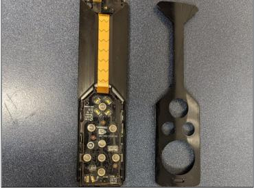
• The Buttons are easily removed. The Volume Touch pad is also seen here; it is attached by glue.
