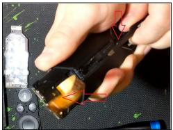
• The Sensor Ribbon is carefully peeled away from the glue. There are two options available to get the battery compartment out. You can either use the Tweezers and push near the ribbon cable or you can use the tweezers to push from the other end inside and under the Sensor place as seen in the picture.
