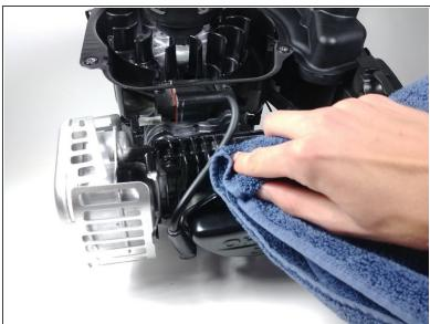
Using compressed air and a rag, clean the heat sink.
