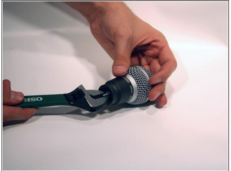
**⚠** Never open the microphone capsule. Attempting to open the capsule will likely result in permanent damage and make the microphone unusable.
