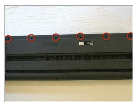
Remove the six 10mm screws at the top of the backplate.
