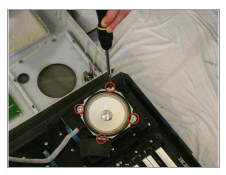
Locate the speaker and remove the four 10mm screws in the corners of the speaker.
