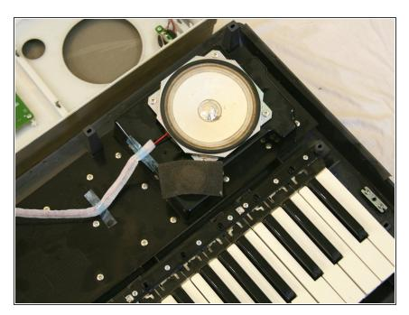
Remove the translucent blue tape that holds the speaker wires to the keyboard.
