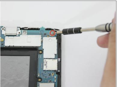
With the Phillips #000 screwdriver, unscrew the four 4.0 mm screw that are holding down the motherboard.
