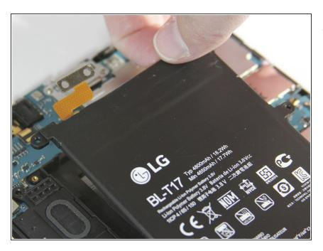
Lift the battery with your fingers and remove it from the device.
