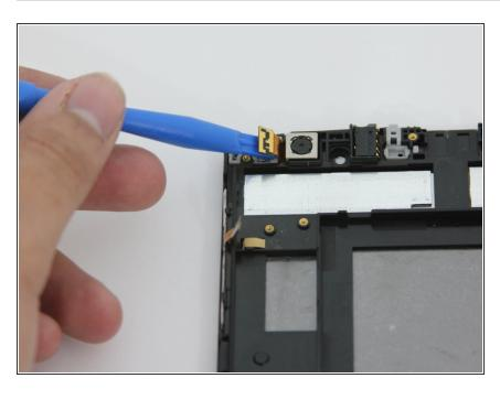
Insert the plastic opening tool under the ribbon connector that is holding the rear-facing camera down and lift it up.
