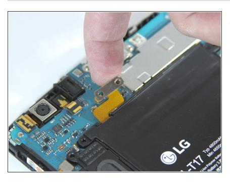
Lift the battery ribbon connector with your finger.
