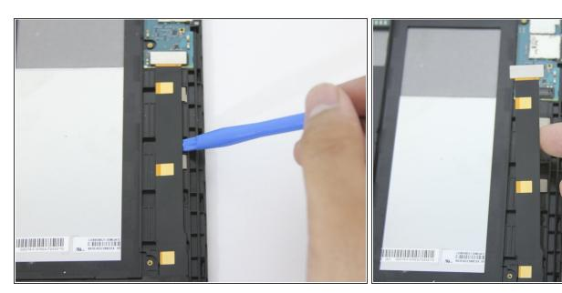
Use a plastic opening tool to lift up the ribbon connector at the bottom of the motherboard.
