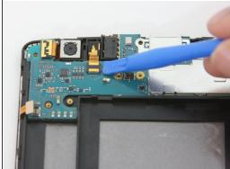
Lift and release the remaining ribbon connectors in the upper left corner of the motherboard with a plastic opening tool.
