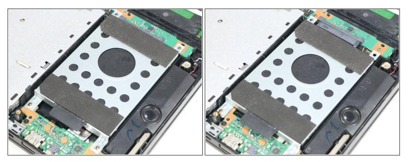
• After removing the four screws, gently push the hard drive downward as shown.
