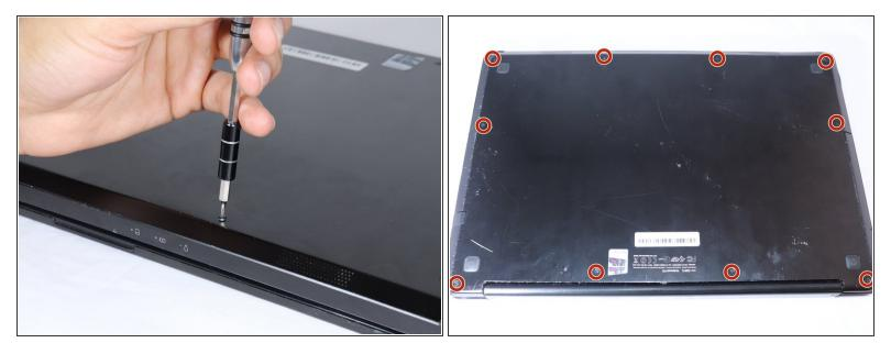
Unscrew the 10 screws around the edge of the back panel. Eight of the screws are 0.0793mm T5, two of them are 0.0793 JIS #0.
