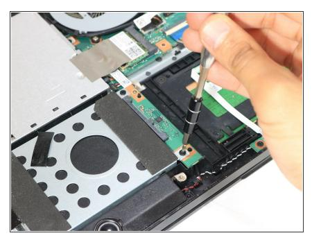
• Using the PH0 and screwdriver from the 54 Bit Driver kit.
