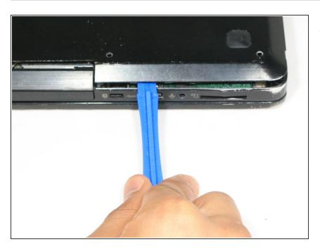
Use the plastic opening tool to pry the back panel off the base of the laptop.
