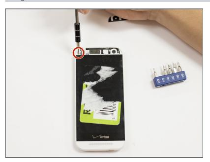
• Take out the single 3mm screw that is on the top left side using a Torx 4 screwdriver.
