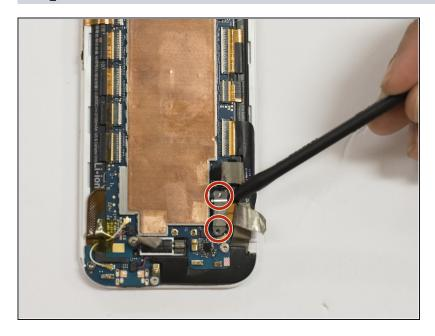
Remove the two 1mm screws at the bottom right of the motherboard using a Phillips #00 screwdriver.
