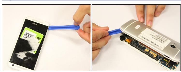
• Use the plastic spudger to pry off the back cover. Place the tool in the SIM card insert and lift the back cover with force. Continue to do this all around the phone.
