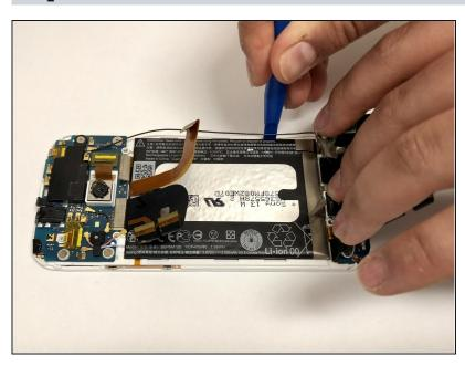
Pull back the ZIF and ribbon connectors and place the plastic opening tool into the indentation between the battery and the frame of the phone. Continue to do this around each side of the battery by gently prying.
