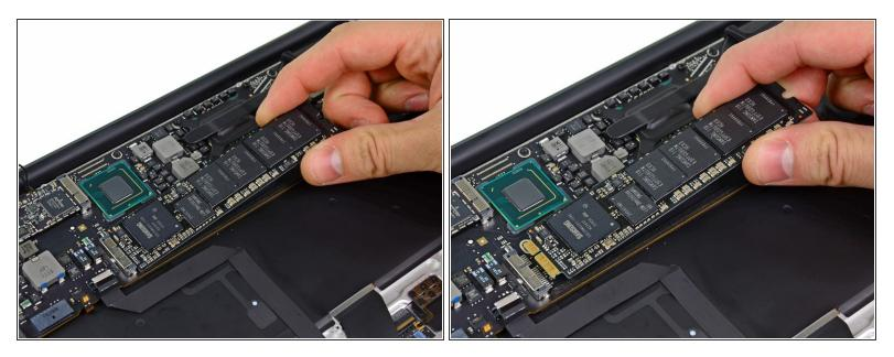
↑ To avoid damaging its socket, do not lift the end of the SSD excessively.
