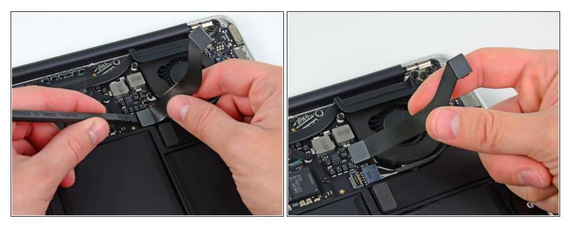
A The following connector has an especially deep socket. Use care when disconnecting it.
