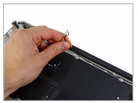
• Gently de-route the antenna cables out of the channel cut into the upper case.
