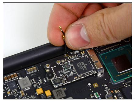
• Gently de-route the antenna cables from the slot cut into the logic board.
