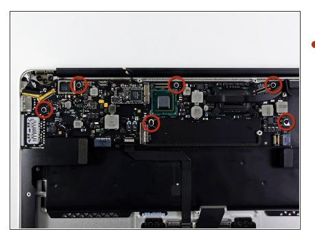
Remove the six 6.3 mm T5 Torx screws securing the logic board to the upper case.
