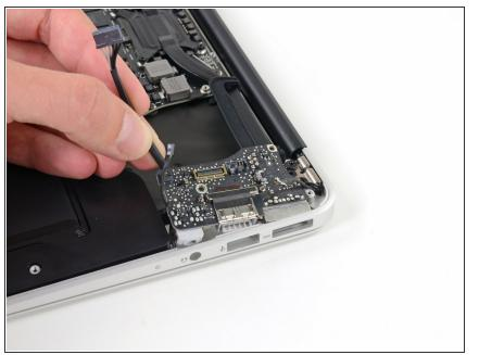
• Carefully lift the I/O board from its edge nearest the logic board and remove it from the upper case.
