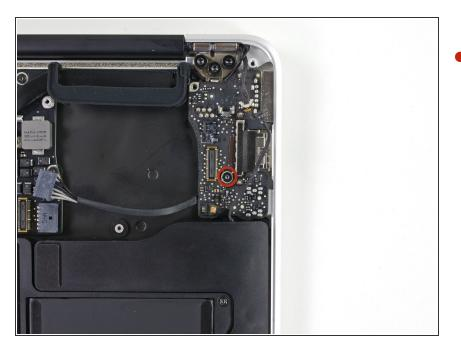
Remove the single 4.0 mm T5 Torx screw securing the I/O board to the upper case.
