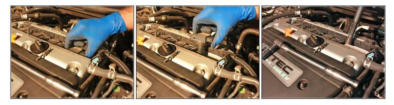
Lift the boot screws out of the spark plug bores.
