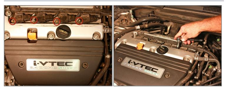
Use a 10 mm hex driver or socket to remove the four spark plug boot screws.
