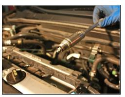
• Pull the plug out of the bore.
