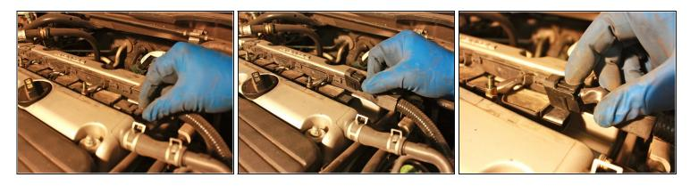
Remove the spark plug wire by pinching the locking tabs on either side of it and pulling it out.
