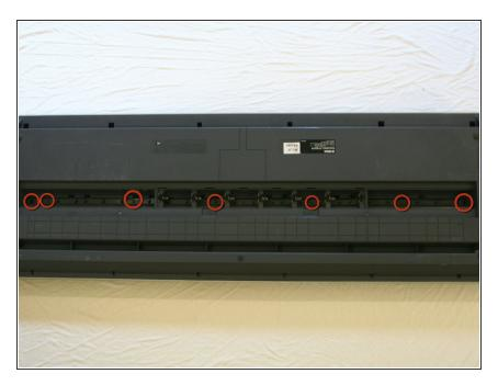
Remove the seven 12mm screws in the middle of the back plate.
