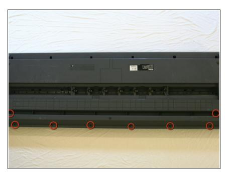
Remove the eight 10mm screws from the side and the bottom of the back plate.
