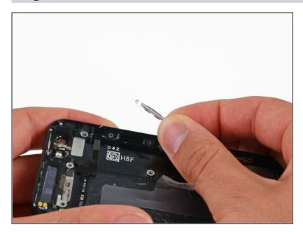
• Remove the four front panel clips from the rear case.
