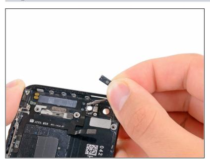
Remove the power button from behind its cover in the rear case.
