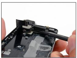
Use the flat end of a spudger to gently pry the Lightning connector and speaker enclosure assembly cables up from the rear case.
