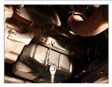
Place the oil drip pan under the drain plug and begin to loosen the drain plug with a 17mm wrench.
