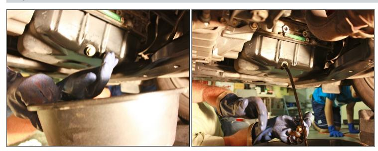
• Loosen drain plug slowly by hand until the bolt is completely removed and oil begins to flow, re-positioning the oil drip pan if needed.
