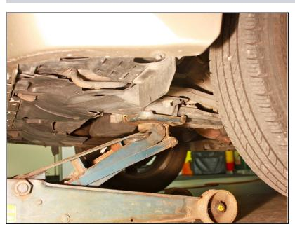
Push downward on the jack's lever to lift the saddle upward so that it contacts the crossmember.
