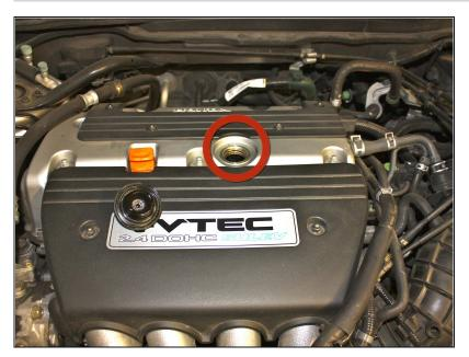
Locate the oil fill cap on top of the engine and unscrew it.
