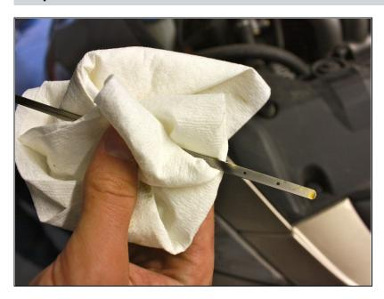
Remove the dipstick and examine the oil levels. The oil level should be between the two dots on the dipstick.
