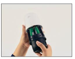
A Removing the lid too quickly could cause you to tear the interconnect cable that attaches the base to the top of the lid.
