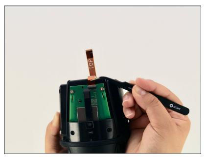
Carefully remove the interconnect cable using a pair of <u>tweezers</u>.
