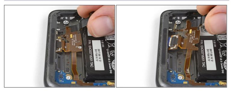
• Gently pull the USB-C port out of its recess in the phone case.
