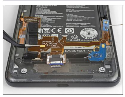
• Lift the charging assembly out of the phone case.
