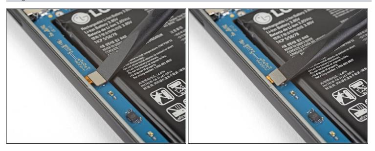
• Use the flat end of a spudger to disconnect the left Active Edge sensor connector.
