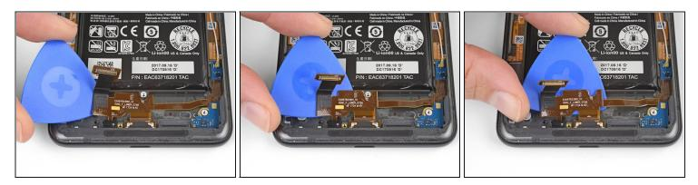
• Starting from the left side, slide an opening pick under the charging assembly flex cable to separate it from the phone case.
