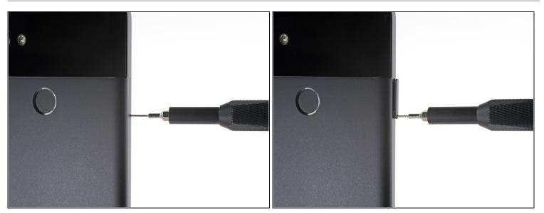
• Insert a SIM card eject tool or a paperclip into the small hole in the SIM card tray, located on the left edge of the phone, opposite of the power and volume buttons.
