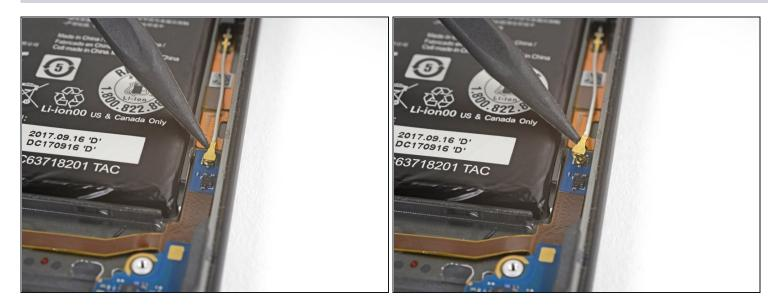
• Use the point of a spudger to disconnect the white antenna cable to the right of the battery.
