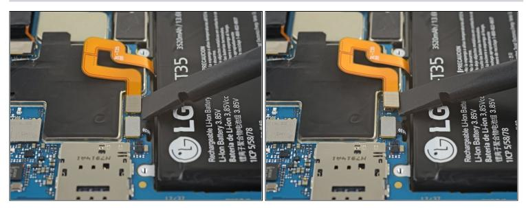
• Use the flat end of a spudger to disconnect the battery connector.
