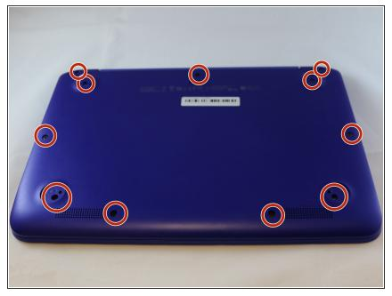
Using the Phillips #1 screwdriver, remove all 11 of the the 5mm screws.
