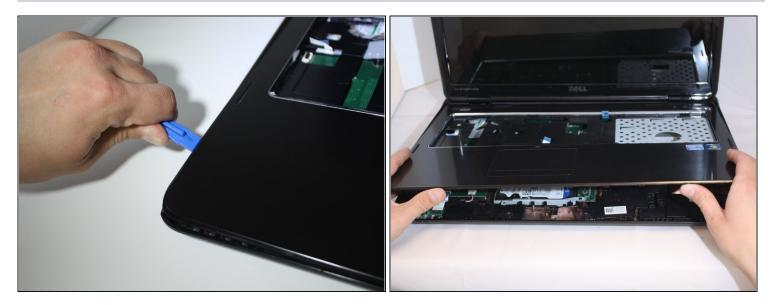
⚠️ Do not proceed without holding the laptop screen/lid for support. The screen is very heavy and may cause the device to fall if not held and supported.
