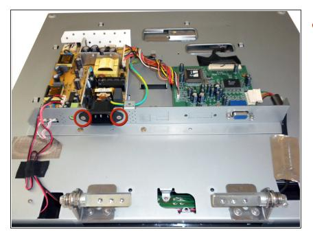
Using a #2 Phillips screwdriver, remove the two 4.72 mm Phillips screws that hold the power adapter in place.
