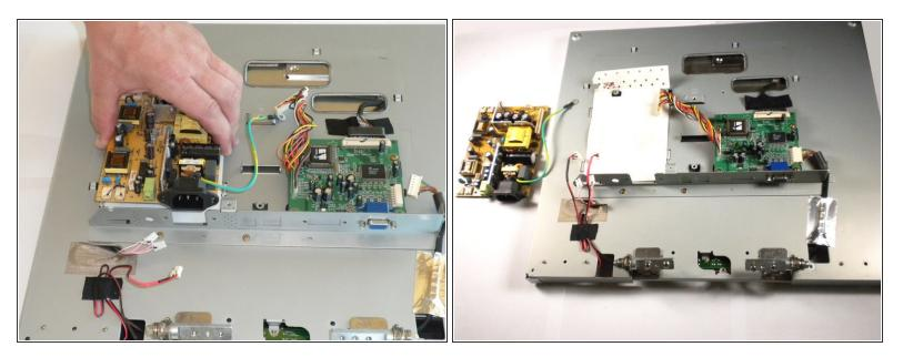
• Lift the power supply unit straight up to remove it from the back panel.
