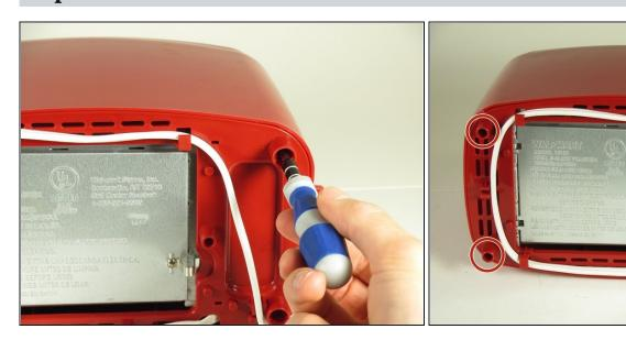
• Use a Phillips #2 screwdriver to remove four 12 mm screws at the base of the toaster shell.
