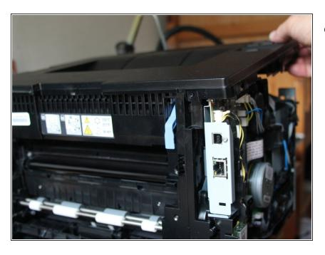
Carefully lift the cover (Attention: cable connection to the display is hanging there) and rack it to the back of the printer (move it back and forth to unhook the locking nipple): unplug the display connector (yellow lines) from the I/O board, unroute the cable and remove the cover.
