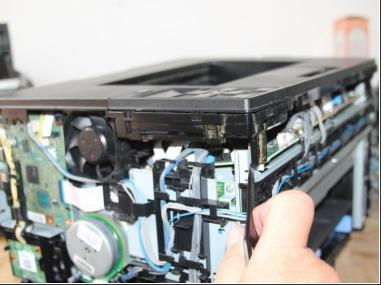
Remove two srews from the front. And to take off the cover leverage remove the tabs diagonally from the front over the latching.
