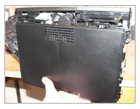
Reposition the printer and hold the disengaged lugs in the disengaged position. Open the rear flap and slide the side panel backwards while moving away from the printer.
