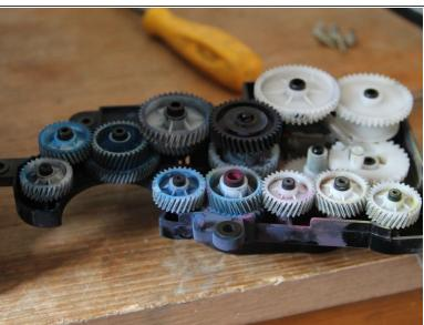
Next, we remove the color control gear (black, large plastic bracket with 15 meshing gears (5 screws have to be loosened).
