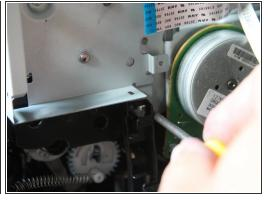
The metal plate under the I/O card (which holds the I/O card) is secured with 3 screws. Remove all 3 screws
