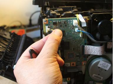
The WLAN card is secured with a screw-> remove it, carefully unplug the WLAN card and remove the WLAN bracket together with the cable
