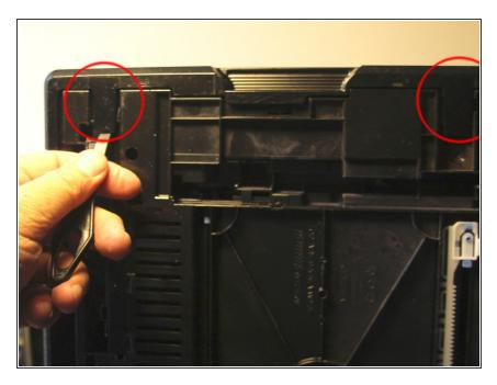
Place the printer on the right side and remove the left side panel (there are 2 lugs under the printer)
