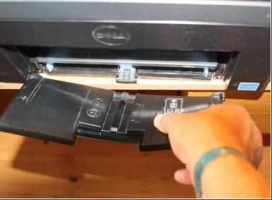
Remove the front paper tray by slightly bending it carefully and angling it to release the peg from the hinge slot.
