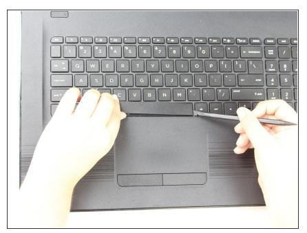
Slide the spudger under the spacebar key.
