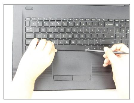
At the edge of the space bay key use a spudger to help with the removal.
