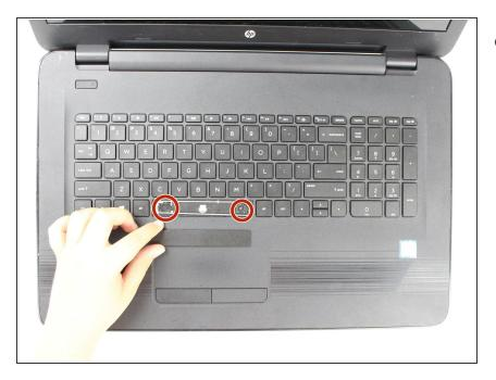
The lower edge of the keyboard has two plastic notches on either side.
