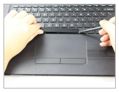
The left side of the spacebar key will start lifting up. At this point you can remove the spacebar key.
