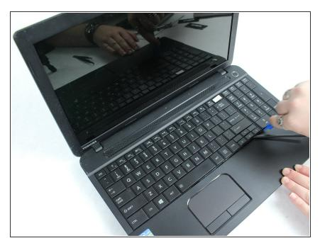
Use the plastic opening tool to remove the keyboard from the laptop.
