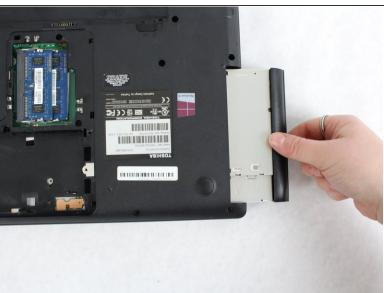
Using a plastic opening tool, pry open the disk drive. Once it has loosened it will pull out.
