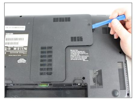
Use the plastic opening tool to pry open the back panel. Make sure to loosen all four sides then lift up.
