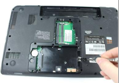
Remove a .5mm screw with a JIS #000 screwdriver.
