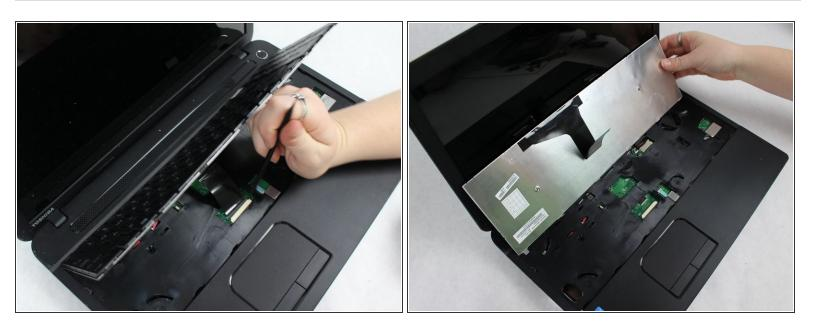
Once the keyboard is popped out, use a spudger to undo the ribbon or flap that attaches the back of the keyboard to the inside base of the laptop.
