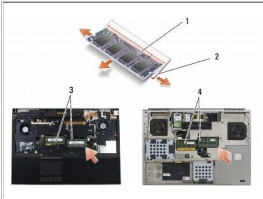
**(i) NOTICE:** To prevent damage to the memory module connector, do not use tools to spread the memory module securing clips.
