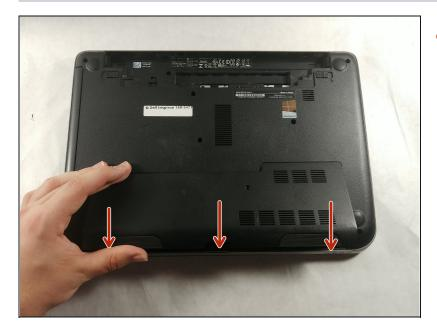
Start by removing the cover that hides all the internal components by sliding it in the direction shown
