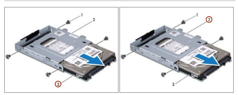
Slide the NEW hard drive into the hard drive cage.
