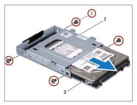
Replace the four screws that secure the hard drive to the hard drive cage.
