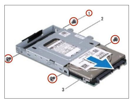
Remove the four screws that secure the hard drive to the hard drive cage.
