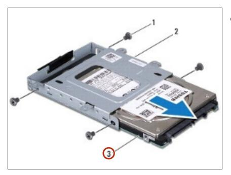
Slide the hard drive out of the hard drive cage.
