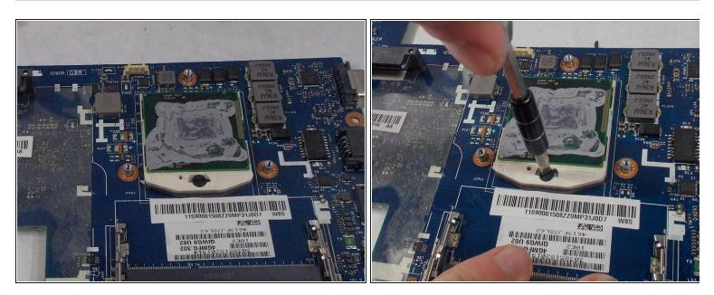
• Using a flathead screwdriver, turn the beige lock to counterclockwise to unlocked.
