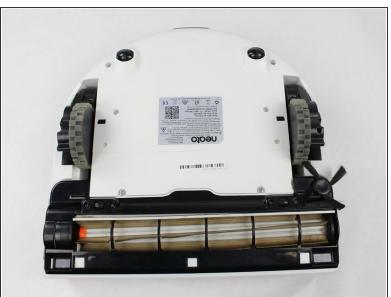
Turn the robot upside down to locate the battery cover.
