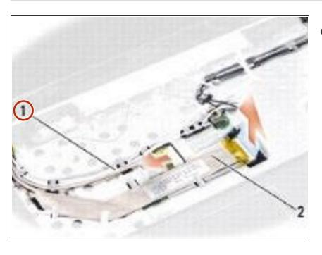
Disconnect the camera cable from the system board connector.
