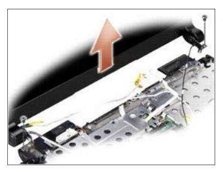
Make note of the cable routing and carefully dislodge the antenna cables and the rest of the cables from their routing guides. Pull the cables away, so that they are clear of the palm rest.
