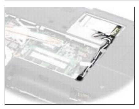
Carefully route the WLAN card antenna cables through their routing guides and connect them to the WLAN card.
