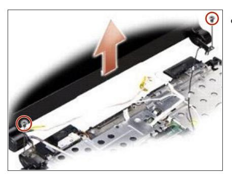
Remove the two M2.5 x 5-mm screws from either side of the display assembly.
