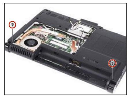
Turn the computer over and replace the two M2.5 x 5-mm screws on the computer base.
