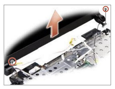
Replace the two M2.5 x 5-mm screws on each side of the display assembly.
