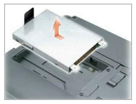
Slide the hard drive carrier away from the screw holes, and then use the tab to lift the hard drive straight up to remove it from the computer.
