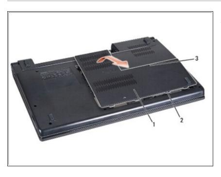
Loosen the three captive screws on the base cover and lift the base cover off the computer at an angle as shown in the figure.
