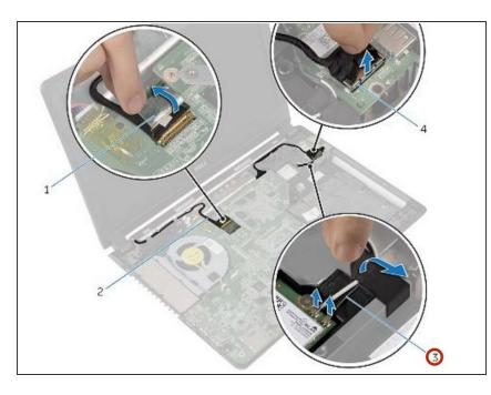
• Disconnect the antenna cables from the wireless card.
