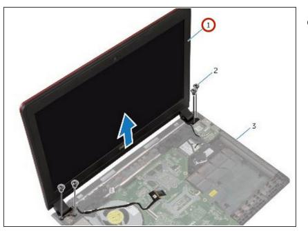
Place the NEW display assembly on the computer base and align the screw holes on the display assembly with the screw holes on the computer base.
