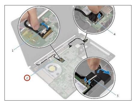
Note the display cable routing and remove the cable from its routing guide.
