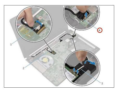
• Connect the I/O-board cable to the I/O board.
