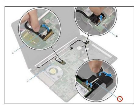
Route the antenna cables through the routing guides on the computer base.
