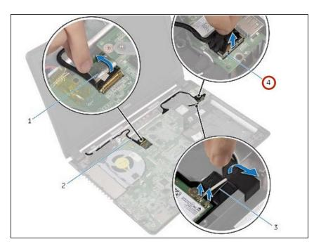
Route the I/O-board cable through the routing guides on the computer base.
