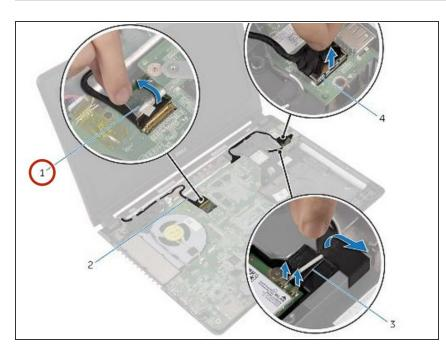
• Peel off the tape that secures the antenna cables to the speaker.
