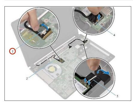
• Adhere the tape securing the antenna cables to the speaker.
