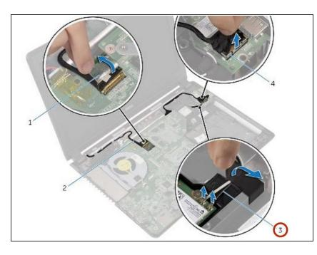
• Connect the antenna cables to the wireless card.
