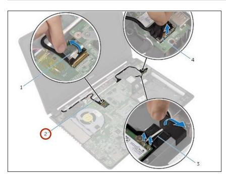
• Route the display cable through the routing guides on the computer base.
