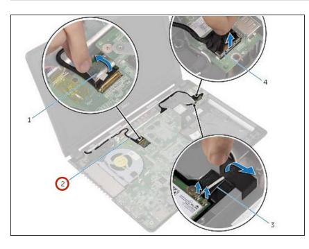
• Connect the display cable to the system board and adhere the tape.
