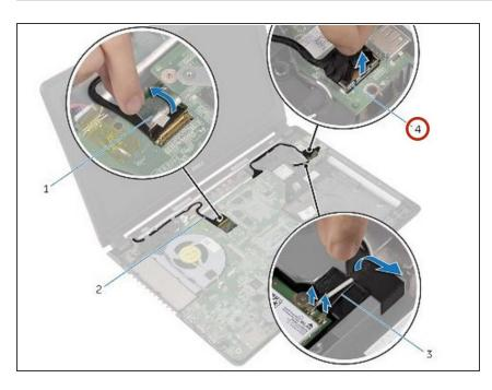
Note the I/O-board cable routing and remove the cable from its routing guide.
