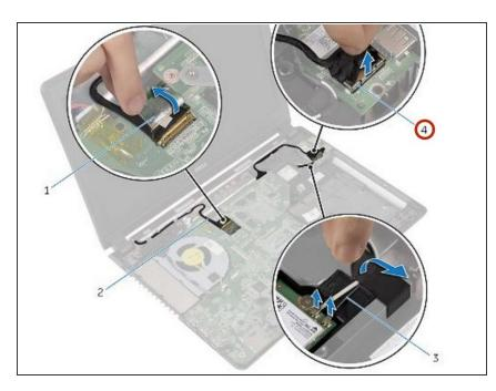
• Using the pull-tab, disconnect the I/O-board cable from the I/O board.
