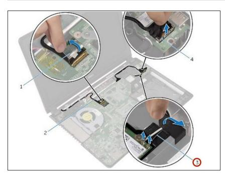
Note the antenna cable routing and remove the cables from their routing guide.
